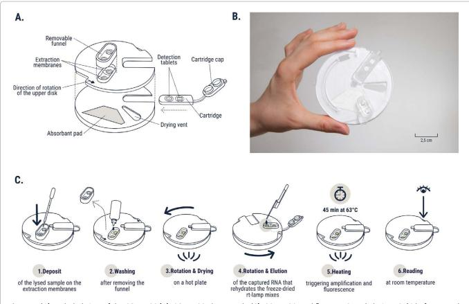
**Figure 1**: (A) Exploded view of the COVIDISC (B). COVIDISC photograph. (C). COVIDISC workflow:  $1 - \text{Sample lysis at 65}^{\circ}\text{C}$  before sample injection. 2 - Washing of the extraction membranes.  $3 - \text{Upper disk rotation and drying at 65}^{\circ}\text{C}$ . 4 - Upper disk rotation and RNA elution. 5 - Upper disk counter- rotation and closing of the cartridge. 6 - 45 min heating and readout at room temperature.
